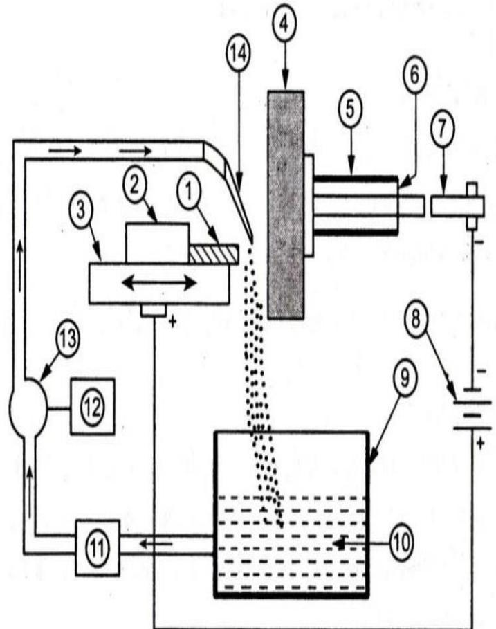
1. Workpiece, 2. Fixture, 3. Work table, 4. Grinding wheel,
