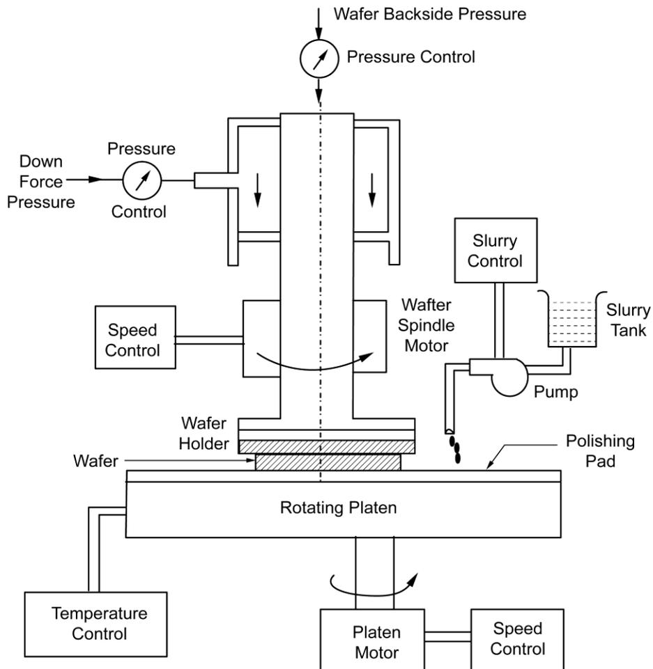
**Fig. Chemo mechanical polishing**
