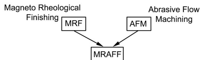
On combining the process, the abrasive medium in magneto rheological abrasive flow finishing can be manipulated and controlled in real time and also it helps in deterministically and selectively abrade the workpiece surfaces.
