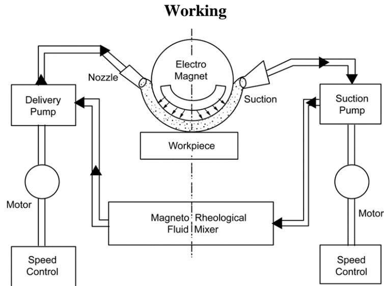
Fig. Magneto rheological fluid circulation system
