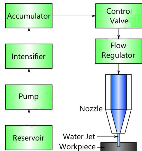
**Reservoir:** It is used for storing water that is to be used in the machining operation.
