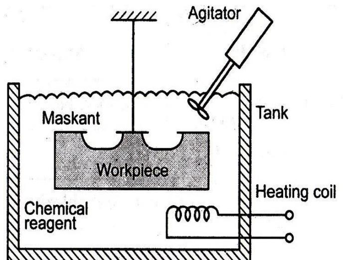
as occurs in corrosion or chemical dissolution of a metal. This controlled chemical dissolution will simultaneously etch all exposed surfaces even though the penetration rates of the material removal may be only 0.0025–0.1 mm/min.
