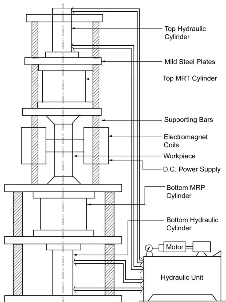
Fig. Magneto rheological abrasive flow finishing
