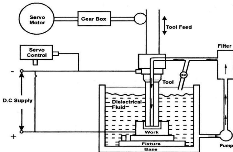
Schematic layout of EDM
