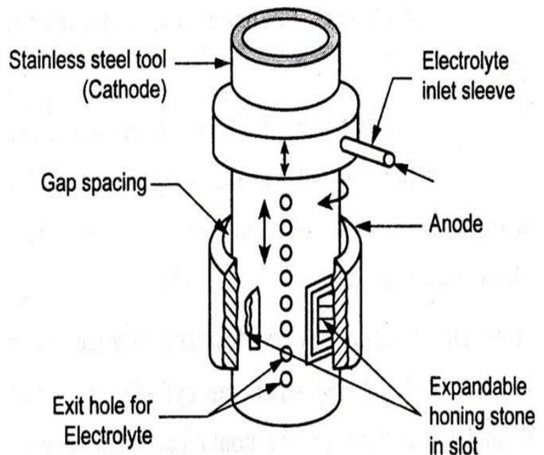
each of the stones exerts equal pressure against the workpiece.
