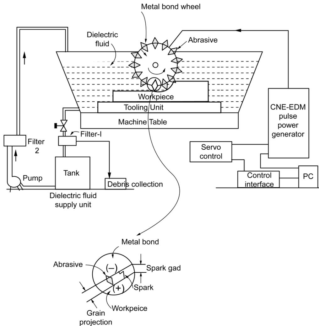
Fig. Schematic Arrangement of Electric Discharge Diamond Grinding
